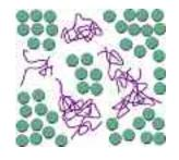
Non-associative polymers thicken by structuring the continuous phase and through chain entanglement. This can stabilize pre-dispersed insolubles by significantly slowing their motion. (*see illustration below*)
